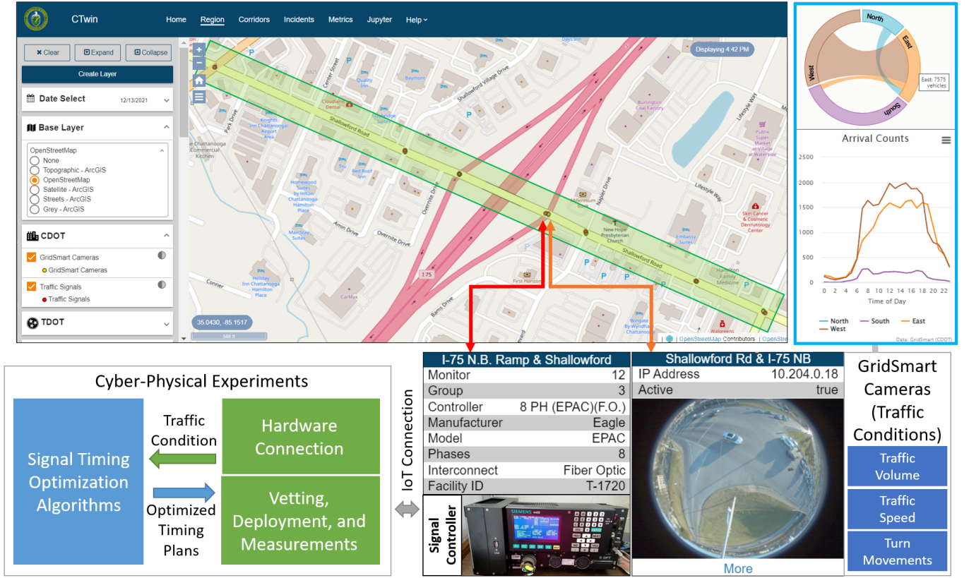
Fig. 6: Cyber-physical control experiments conducted through the CTwin's cyberinfrastructure: Connecting traffic light controller at intersections with signal timing optimization algorithms.
